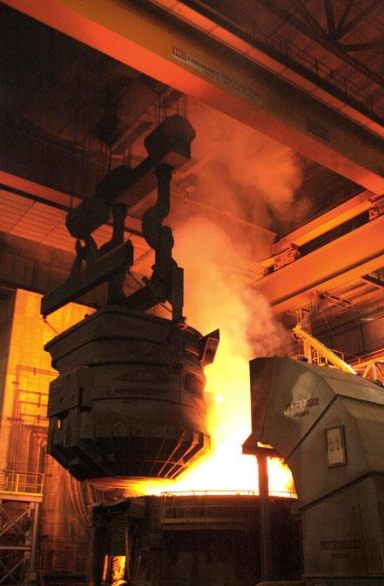
Steel Making Shop – Charging and Ladle
