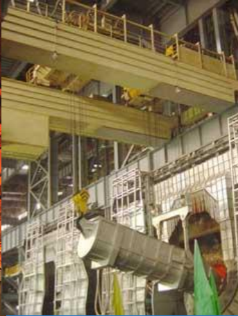
Steel Making Shop – Charging and Ladle
