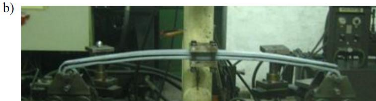
Figure 2. a) Rotating bending test specimen, b) Example of the spring test setting
