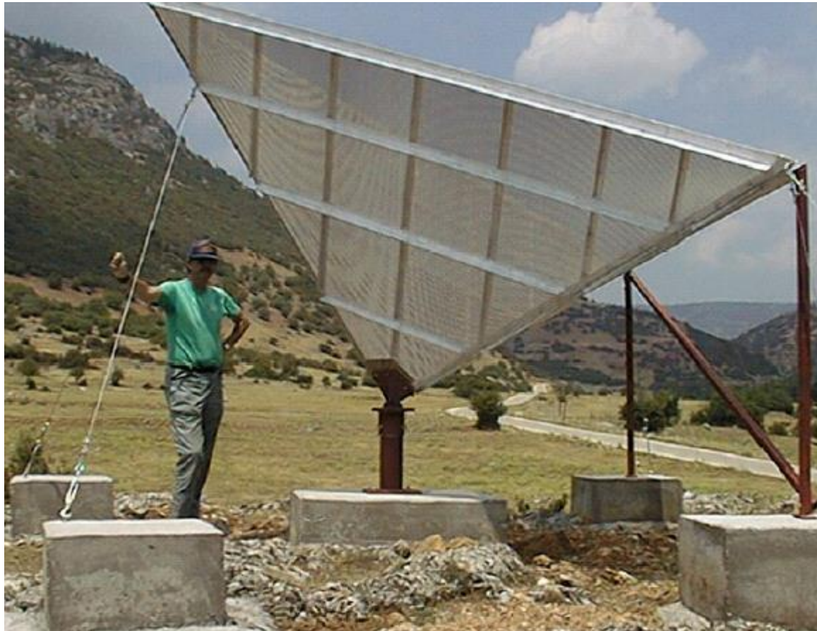
Example of final corner reflector design for the SNAP program as installed in the field.
